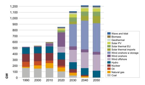
Figure 25: Electric generation capacity in the Mitigation scenario
